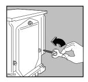
Remove the polystyrene block from the bottom of the machine.
